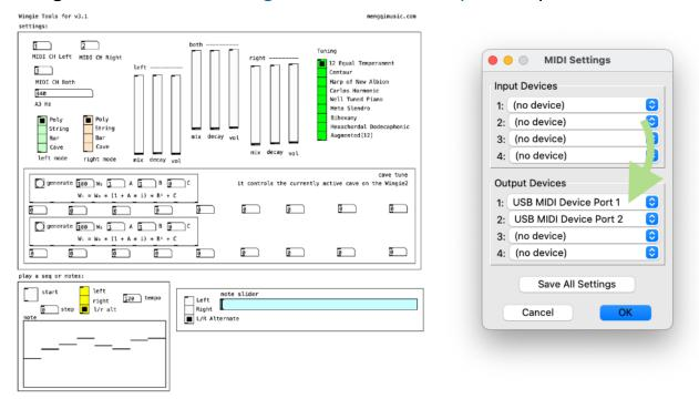
In the "Media / MIDI Settings" menu, select the MIDI port connected to Wingie under "Output Devices" A large frequency jump will result in loud output. Make sure to turn down Volume & Decay before adjustment
